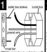
ATTACH cross bar to outlet box with outlet box screws (8-32 x 1/2, 2 slotted screws provided).
