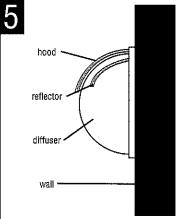
Hood is to be placed above reflector as shown.
