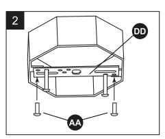
2. Attach crossbar (DD) to outlet box (not included) using short screws (AA).
