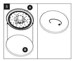
**5.** Align the tabs on fixture pan (A) with the channels on diffuser (B), then insert diffuser into fixture pan. Carefully twist the diffuser (B) clockwise until secure.
