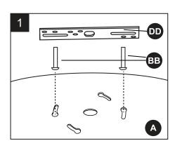
1. Align two of the threaded holes on crossbar (DD) over one set of keyhole slots on the fixture pan (A). From the inside of fixture pan (A), insert long screws (BB) into aligned holes, leaving about 1 in. of space between the screw heads and crossbar (DD).
