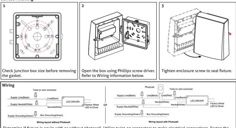
Determine if fixture is equip with or without photocell. Utilize twist-on connectors to make electrical connections. Fasten the wires by the provided cable tie.
