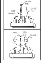
**STEP 1.** Insert wires into Quick connector, black to black and white to white, attach ground wire to ground screw in recessed can.
