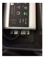
Carefully relocate the driver and wires to get access to the (2) hex bolts.
