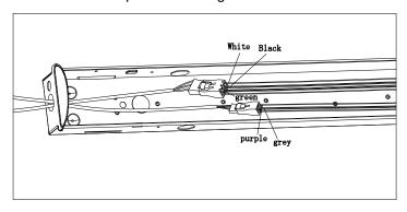
6.Install the module board and lampshade
