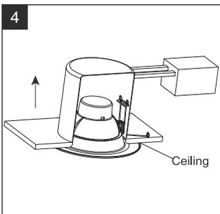
4. Squeeze torsion springs together as shown and install into torsion spring brackets inside recessed housing. Carefully route wires into fixture and push recessed kit up flush to ceiling surface.
