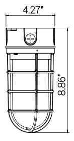
ConstructionFixture MaterialAluminumFixture FinishMetallicLens MaterialGlassLens FinishClearShapeRoundMountingSurface
