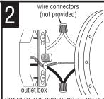
CONNECT THE WIRES. NOTE: Attach the black fixture wire to black supply wire, the white fixture wire to white supply wire and bare or green fixture wire to around supply wire. Do not mix them up. Use wire connectors (not provided).
