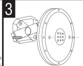
and green fixture ground wire to ground screws and secure in place with thumb THREAD fixture mounting screws wire in outlet box. NOTE: wire connectors nuts (provided). Fixture may be mounted not provided. NEVER CONNECT GREEN to ceiling or wall. The photo sensor or ATTACH cross bar to outlet box with FIXTURE GROUND TO BLACK OR WHITE knock out must be orientated down when the fixture is mounted to a wall.
