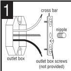
ATTACH CROSS BAR to outlet box with outlet box screws (not provided) THREAD NIPPLE into cross bar. Adjust nipple to proper height for mounting fixture.
