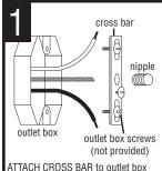
with outlet box screws (not provided) THREAD NIPPLE into cross bar. Adjust nipple to proper height for mounting fixture.
