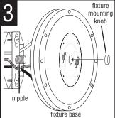
POSITION THE FIXTURE BASE over the nipple and secure into place with the fixture mounting knob.
