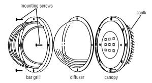
PLACE DIFFUSER ON CANOPY. Then place bar grill or frame over diffuser and attach to canopy with mounting screws. (8-32x1/2, 4 combination head screws provided)
