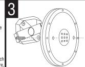
and green fixture ground wire to ground screws and secure in place with thumb wire in outlet box. NOTE: wire connectors nuts (provided). Fixture may be mounted not provided. NEVER CONNECT GREEN to ceiling or wall. The photo sensor or knock out must be orientated down when the fixture is mounted to a wall
