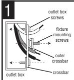
THREAD fixture mounting screws (provided) into outer cross bar. outlet box screws (not provided).
