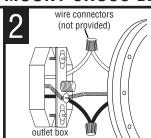
CONNECT THE WIRES. NOTE: Attach the black fixture wire to black supply wire, the white fixture wire to white supply wire and bare or green fixture wire to ground supply wire. Do not mix them up. Use wire connectors (not provided).
