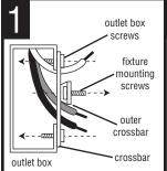
(provided) into outer cross bar. outlet box screws (not provided).
