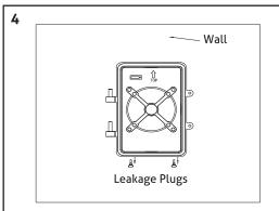
Drill holes according to the size of junction box. Use the level bubble to level the conver and fix it to a sturdy wall. Remove the 2 leakage plugs.
