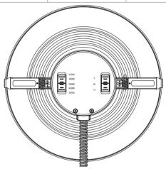
Sunlite's wattage and CCT selector commercial round LED recessed downlight fixture, allows for selecting between power and light temperature settings to match a wide range of applications. With a Color Rendering Index(CRI) of 90, one can expect objects to display excellent color accuracy.
