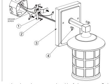
E. Pull on each wire lead to make sure connections are secure. Make certain no bare wires are exposed outside of wire connectors. Tuck all connections neatly into the junction box.
