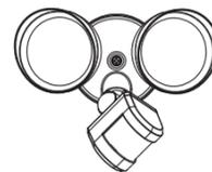
The sensor can clockwise rotate max 45°
